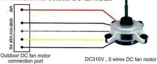
Diagram of DC fan motor connection port:
